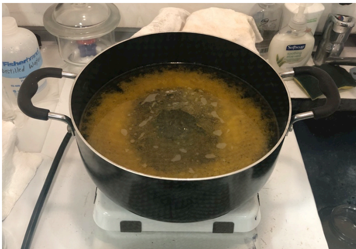
Figure 9. Boiling linseed oil in water on a hot plate.
