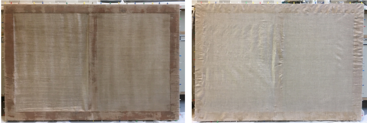
Test canvas before (left) and after drying (right). The left half of the canvas was sized with 7% gelatin, and the right half with 7% rabbit skin glue.
