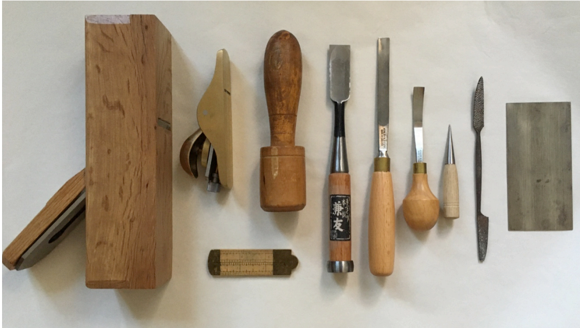
Figure 5. Tools used (left to right): block plane, sole plane, ruler, mallet, flat chisel, straight gouge, curved gouge, awl, rasp, and cabinet scraper
