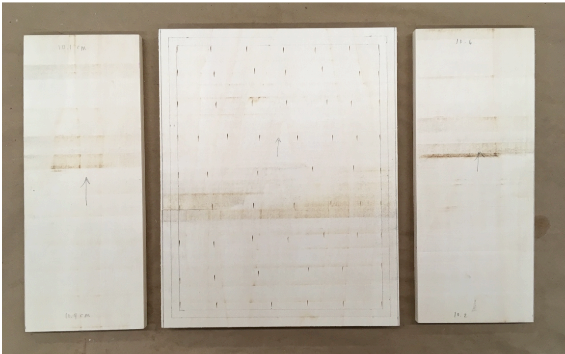
Figure 4. The panels with the central panel showing the marks to set the depth of the recess (Photo: author)
