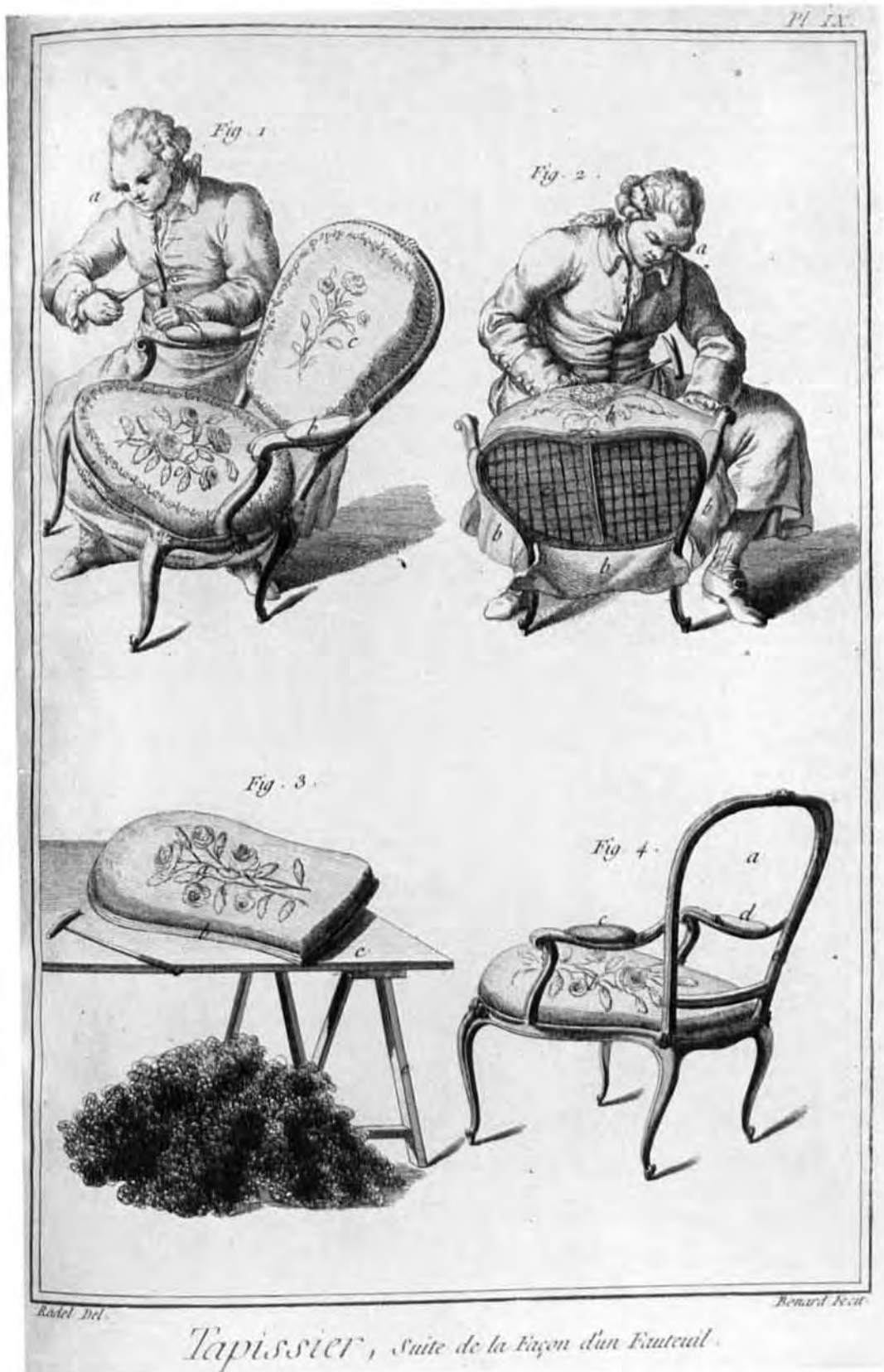
viii. Upholstering an armchair. From Diderot's Encyclopédie . . . Recueil de planches . . . vol. IX, 1771
